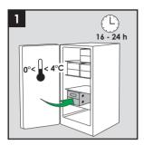
The appliance is not designed to cool down kegs. Therefore please make sure that the kegs are precooled in a refrigerator or cold room for at least 16-24 hours before use (Figure 1). Please therefore ensure that the required kegs are stored in corresponding cooling units or cold stores in good time prior to use.
