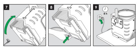
Now connect the power cord to the power supply. (See 3.3 Electrical Installation).
