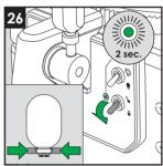
The keg is now locked and the pump audibly generates positive pressure in the keg. Once the pump switches off after around 30 seconds, the beer is cooled actively. The cooling fan is the only thing that can now be heard.
